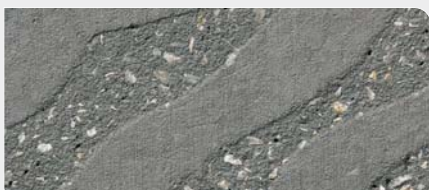
Sand Blasting Ideal for embedding symbols, logos or unique patterns, this method removes the top layer of the cured concrete to reveal a sandy finish.
