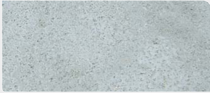
Rock Salt A pitted or 'volcanic stone' look is created with CCS imprint mats or by adding 10mm grains of rock salt to the wet surface.
